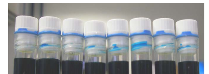
Fig. 4: High risk of carryover – unfavorable sample distribution – when using tubes with internal threading
